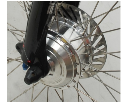
A 250 watt front hub motor
